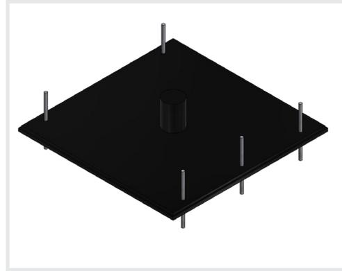
*This is the base or mount (top view) and shows molded-in terminals and threaded insert; the lip or ledge around the outside is where the sleeve will rest, ensuring proper mating between sleeve and base*
