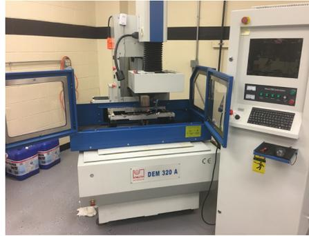
**DEM 320A - CNC Electric Discharge Machine**
