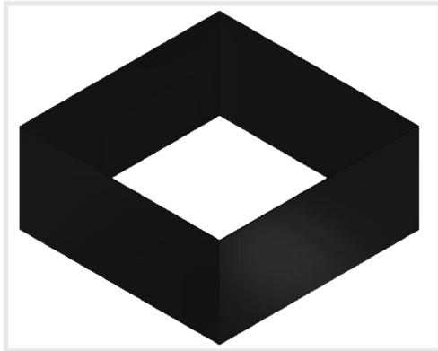
*This is the sleeve; this is used as a container to shape and hold the epoxy encapsulant*
