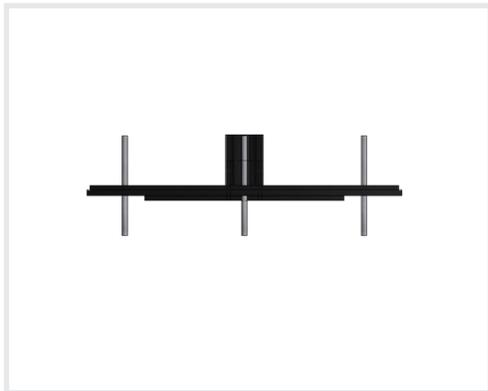
*This is the base or mount (side view) and shows the standoff designed-in as part of the molded configuration.*
