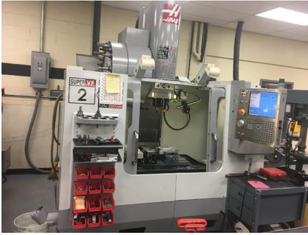
**HAAS VF2SS – Vertical Machining Center**
